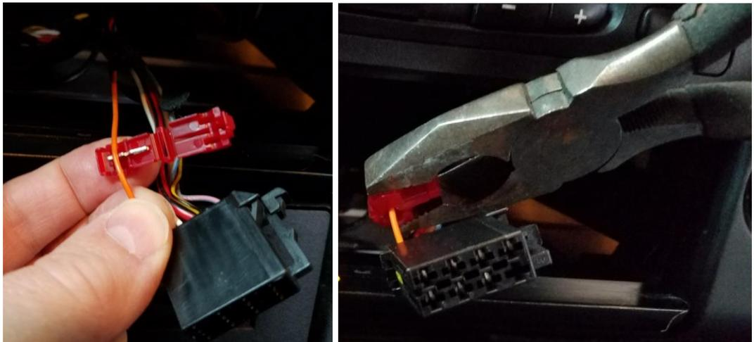
**Note:** Offset the two T-Taps – so one is closer to black connector than the other.
